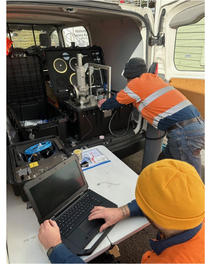
Workshop and Site Mobile Computerised Pressure Relief Valve Testing
